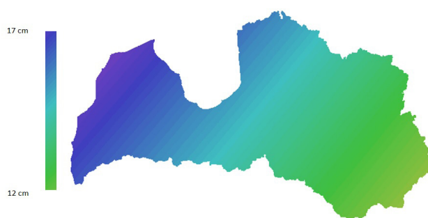
Fig. 8. Data conversion algorithm from BAS-77 to LAS-2000.5 [made by the authors, visualised by the Trimble Business Center].
