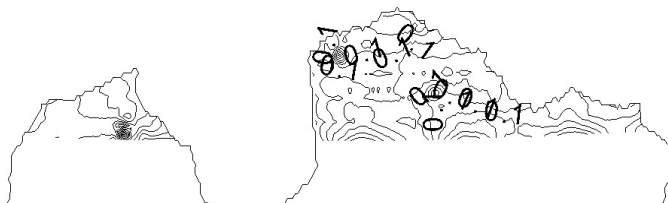
Fig. 6. Differences between q-geoid model EST_GEOID2003 and LV14 (version 3) in Latvia. Contour interval is 0.2 m [made by the authors, visualised by the Trimble Business Center].
