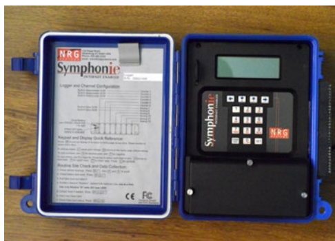
Fig. 1. Registration unit LOGGER Symphonie 9200 for recoding data from sensors of wind speed NRG #40, vane NRG #200, temperature NRG #110s and air pressure NRG BR-20.
