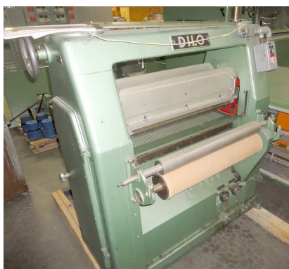
Fig. 3. Laboratory needle loom with one needle board down stroke DILO LBM 6 (600 mm working width, 2000–3000 needles/m., 3000 strokes/min) [15], [16].
