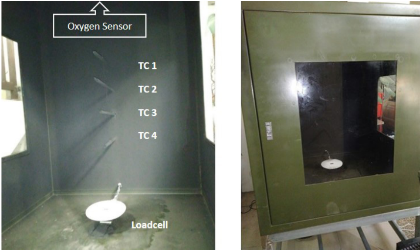
Fig. 1. Schematic and position of sensors inside confined compartment.
