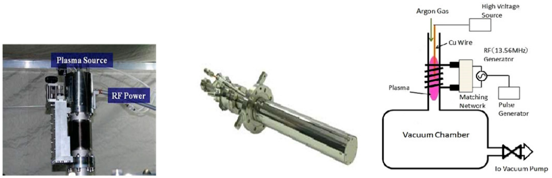
Fig. 8. RF discharge tube and a schematic diagram of the experimental setup of the source with an RF generator (13.56 MHz).
