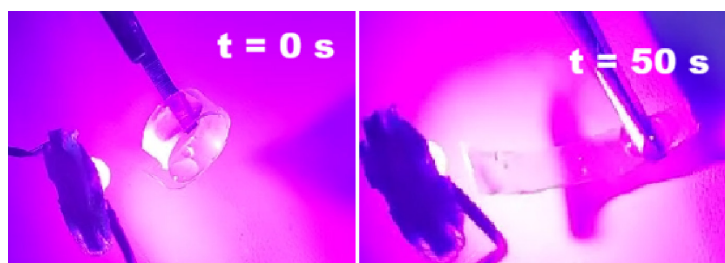
Fig. 5. Unfolding of the shape-memory PU/AgNP composite under 420 nm light stimulus; rolled polymer ( t = 0s ), unrolled polymer ( t = 50s ).
