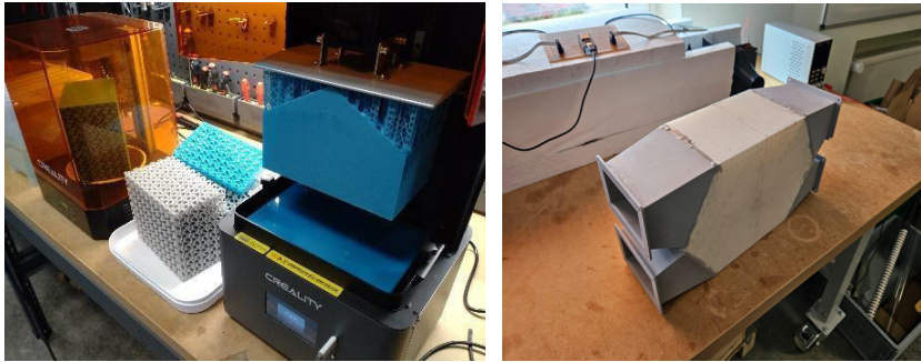
Fig. 5. Heat exchangers printed by UV LCD method.
