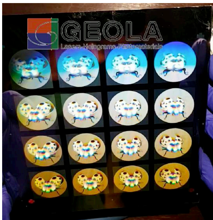
Fig. 13. For comparison this is a hologram of the data of Fig. 9, produced on a DIWO-6 machine.
