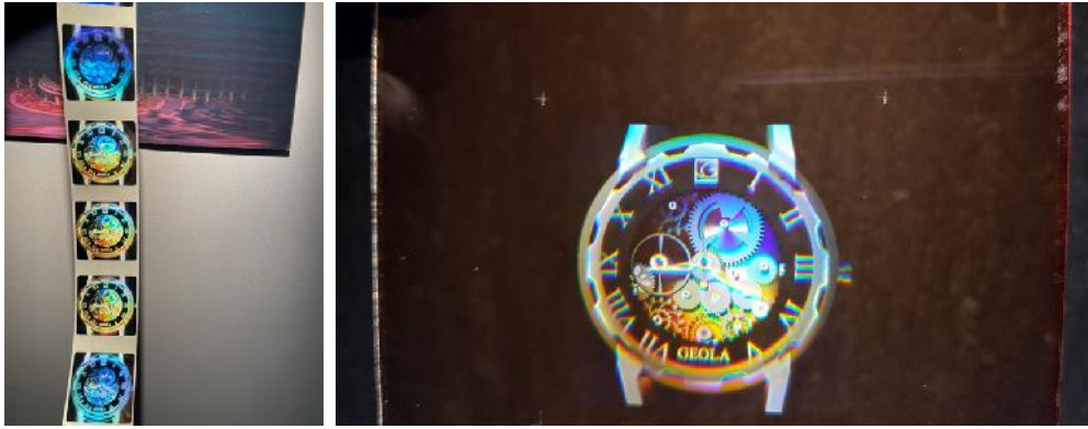
Fig. 5. Full-Parallax Optically-Variable Hologram Labels (Left) and Master (Right). Digital DWDH Master made using DIWO-6 originator on photoresist.
