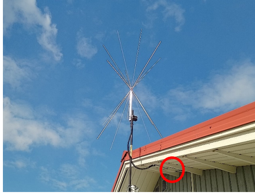
Fig. 3. Omni-directional e-Callisto antenna in Siuntio, Finland. LNA (low-noise amplifier) is located under the eaves (marked with the red circle). The instrument has been operational since April 2023, and since that already tens of solar radio bursts have been detected.
