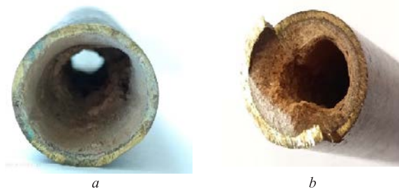
Fig. 1. Photos of a cross section of heat exchange pipes with scale deposits: (a) – condenser pipe, d = 28\text{ mm} ; (b) – peak boiler pipe, d = 19\text{ mm} .
