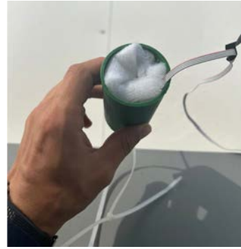
Fig. 4. CO 2 sensor outside installation improvement.
