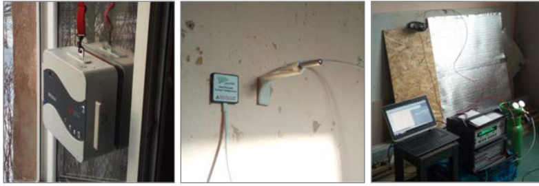
Fig. 5. Measurements of thermal transmittance and air change rate.
