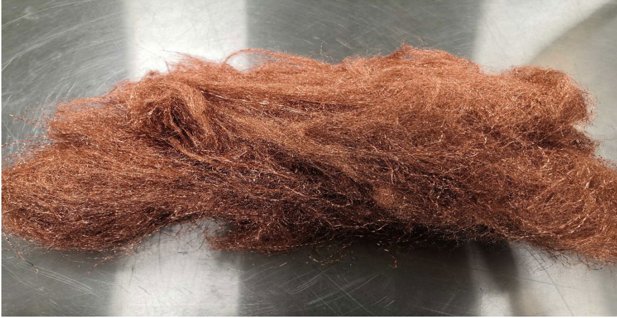
Fig. 2. Copper yarn with continuous 20 thick filament.
