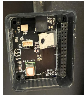
Fig. 1. M5Stack add-on for the CO 2 measurements.
