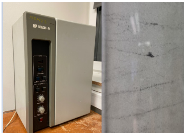
Fig. 1. Ultrasonic mixer (left) and uneven distribution of CNT within Ti-6Al-4V powder (right).
