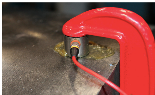
Fig. 5. AE sensor installation method.
