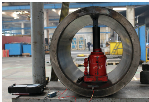
Fig. 4. Installation diagram of the tensile loading device.
