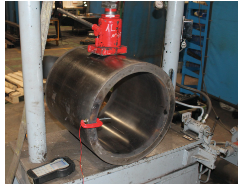
Fig. 6. Installation diagram of the compressive loading device.
