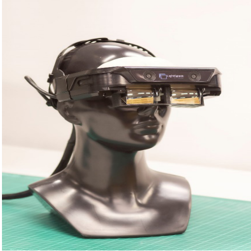
Fig. 1. The multifocal HMD prototype system used for tracking experiments.
