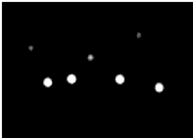
Fig. 3. Comparison of reflectivity as detected by Atracsys FusionTrack 500 for passive fiducials: out of package (bottom row) and after extended handling (top row).
