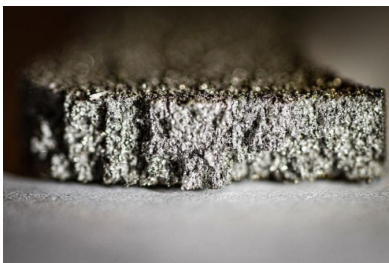
Fig. 8. Zoomed-in photos of broken test samples illustrating the breakage line and surfaces.
