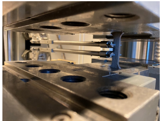
Fig. 5. Tensile strength test setup with an extensometer attached to the test sample.
