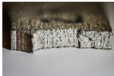
Fig. 8. Zoomed-in photos of broken test samples illustrating the breakage line and surfaces.
