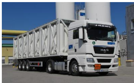
Fig. 4. Containerised hydrogen tubes mounted on a trailer for the transport of hydrogen in central Europe (Co. Linde) [14].
