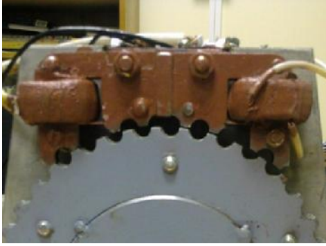
Fig. 1. An experimental model of a generator with a radial arrangement of the magnet and armature windings above the rotor teeth.
