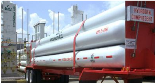
Fig. 5. Example of a large trailer with tank pressure of 25 MPa, per tube, with a total weight of 560 kg of hydrogen [15].
