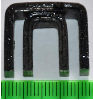
Fig. 14. One section of OMC with two pairs of teeth from laminated steel, size scale in mm.
