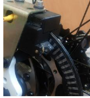
Fig. 11. Placement of the axial generator inductor on the bike frame and the plastic strip of the magnetic flux switch with toggle switches on the steel disc.
