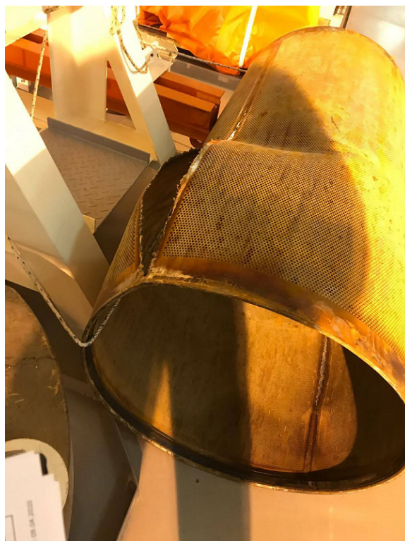
Fig. 1. Failed screen filter after 6-month service under real conditions.
