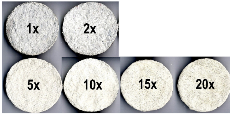
Fig. 2. Examples of specimen groups 2–7. Specimens covered with casein colour and the number of paint layers.
