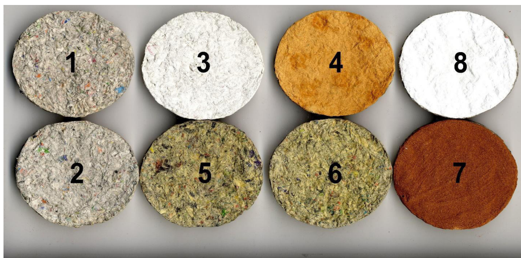
Fig. 1. Examples of specimen groups: 1 – unpainted, 2 – casein primer, 3 – casein paint, 4 – tinted casein colour, 5 – linseed oil paint, 6 – egg oil tempera, 7 – clay colour, 8 – alkyd paint Akrit 7.
