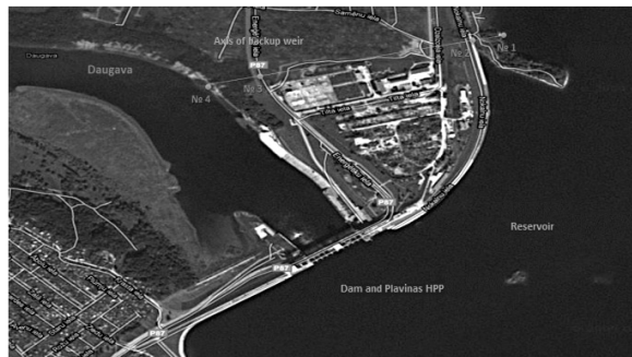
Fig. 4. Optimal deployment of the emergency spillways of Plavinas HPP [14].
