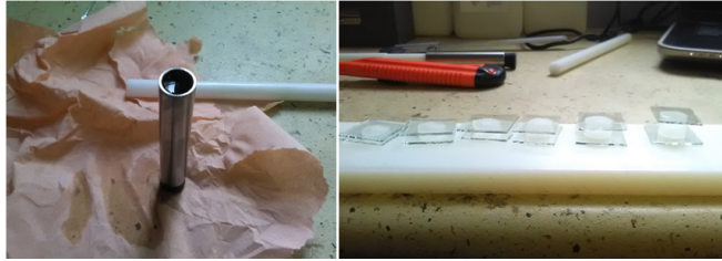
Fig. 2. Extruder with samples of various thicknesses.
